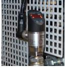
Overpressure Safety Gauge with divider
